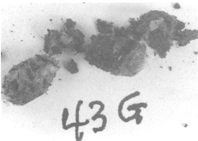
FIG. 1—Two cocoons and other nest debris of Osmia gaudiosa extracted from the fuel control unit of the airplane wreckage. Cocoon length approximately 10 mm.
