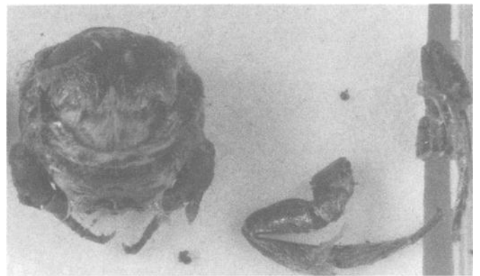
FIG. 3—Thorax and legs of Ashmeadiella sp., from the fuel control unit of the airplane wreckage.
