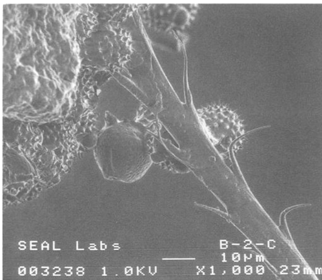
FIG. 5—Scanning electron micrograph of branched hair attached to clump of pollen from B2 elbow. For explanation, see text.
